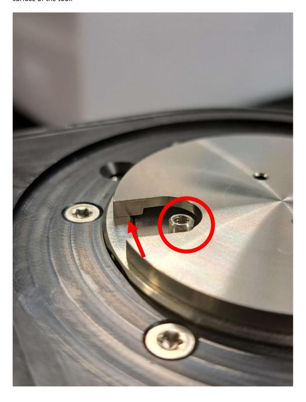
8- After these adjustments, put the two rods in the holes and make sure the rods have touched the bottom of the capsule. Then measure the protrusions using a caliper. The protrusions must be  $10 \text{ mm} \pm 0.15 \text{ mm}$ .
