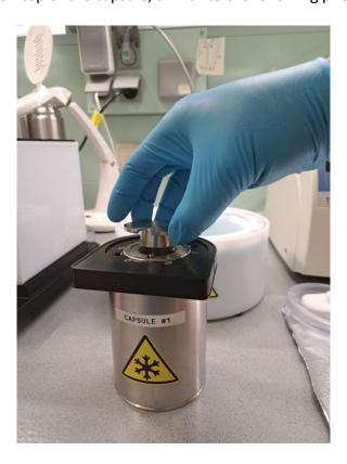
6- Without the cassette, you must be able to turn the tool freely and the pin shall not stop it. Note: it is preferred to adjust the pin as high as possible as when the capsule cools down, the pin shrinks. Indeed, the tool must be fully in contact with the flange of the capsule.
