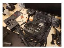
We do recommend testing the system outside of the case prior to assembly to identify any faulty components since re-plugging components is significantly easier prior to mounting.
