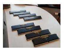
One consideration is that with a four graphics card setup, one requires more system memory than the previous recommended 64 GB. Ideally it would be desirable to fully fill the system with 128 GB of memory, but we have experienced difficulties getting 128 GB of memory to be detected by the operating system, or getting the system to turn on at all. We found that 96 GB to be sufficient for most cases, and would recommend this as a starter.
