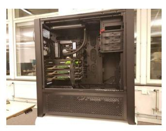
The TR1950X is the flagship CPU from AMD this year. We have incorporated this into our high-end workstation, equipped with four GTX1080Tis and three NVMe M.2 SSDs (one for the operating system, and two in RAID0 as scratch space).
